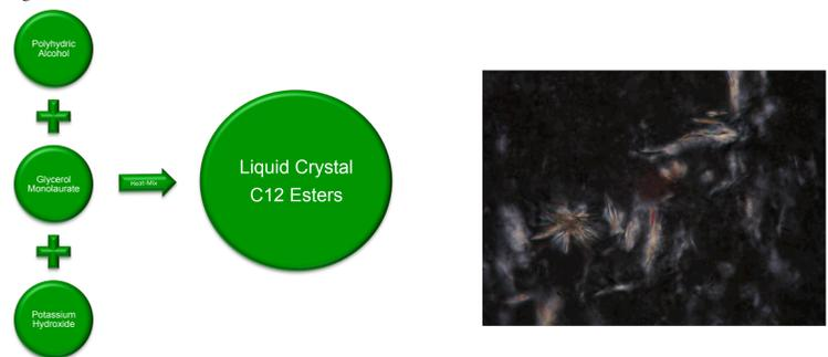
Fig. 1. A. GML, in the presence of a polyhydric alcohol such as propylene glycol or polyglyceryl-2, when heated with the alkali catalyst potassium hydroxide results in the partial saponification and transesterification of GML to the corresponding esters.
